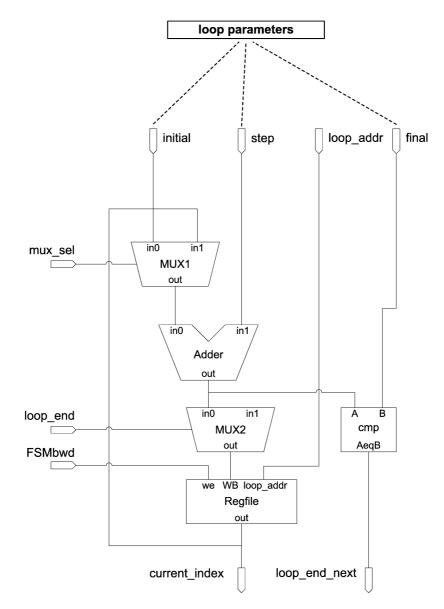
Figure 5. for\_structure\_unit block diagram
