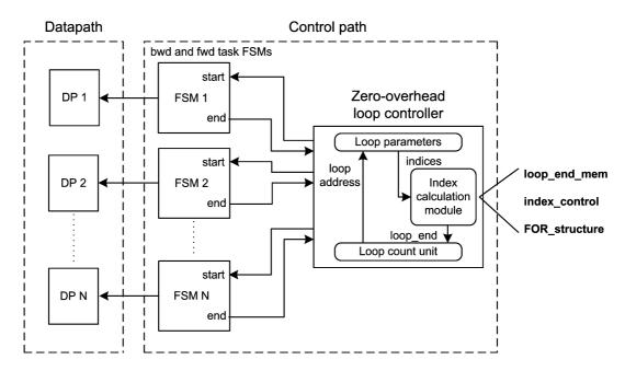
Figure 2. General template of the proposed architecture for implementing multimedia algorithms
