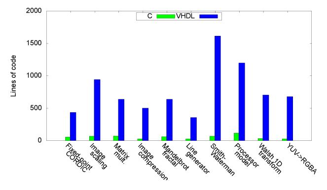
For these ten algorithms, ANSI C code is passed to HercuLeS HLS (http://www.nkavvadias.com/hercules/). At the end of the flow, other things apart, we get the synthesizable RTL VHDL for the given C code. By measuring the VHDL-to-C ratio of useful lines of code (no comments etc), a 7.8x to 25.15x variation with an average of about 15 times (15.4x) is obtained.
